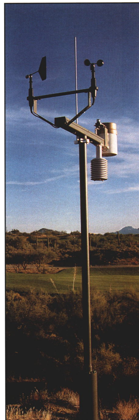
On-site weather stations are often integrated with computer software that can automatically adjust operating times of irrigation sprinklers.
