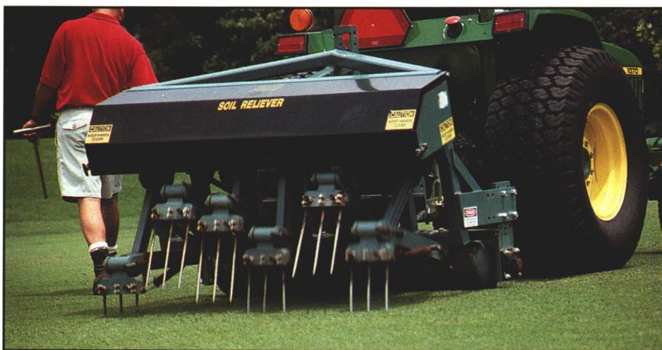
Root zone modification programs normally target the top few inches of the soil profile with shallow-tine aerification. A key benefit of machines like the Verti-Drain or Soil Reliever is fracturing in the lower soil profile.
