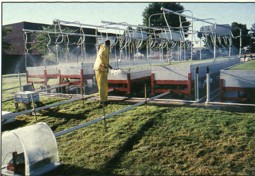
The research greens are constructed from 4-foot by 24-foot wooden boxes. The support legs are blocked for slope adjustment, rain simulators are located overhead, and tipping bucket rain gauges are attached to the drainage outflow lines to allow for the measurement of water output.
