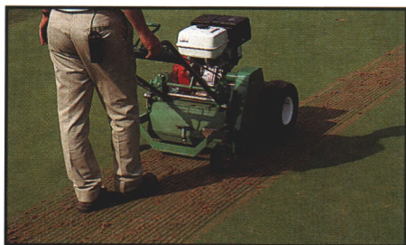
Dethatching removes organic matter and improves oxygen flow to the rootzone.
