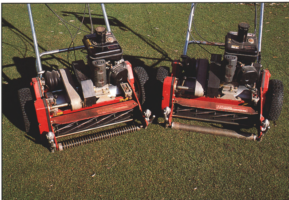
Walk-behind mowers equipped with solid front rollers are recommended to minimize stress to the immature stand of bentgrass during grow-in, especially along the perimeter of the green where the constant turning of grooved rollers usually injures turf.
