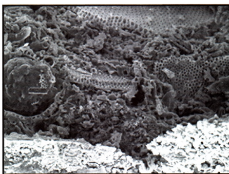
Diatomaceous earth contains many small diatoms that possess a large network of internal pores.
