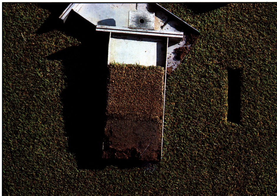
By regularly topdressing the approach areas, a green-type profile can be established over time.
