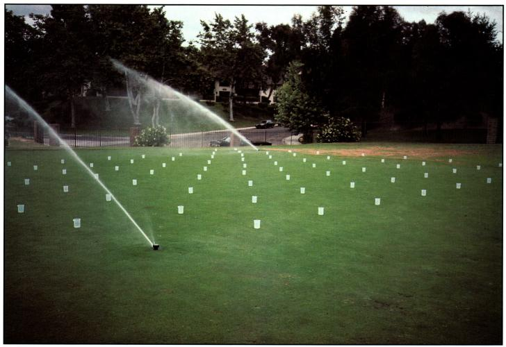
Performing a catch-can test provides data on nozzle and sprinkler performance as it relates to application uniformity.
