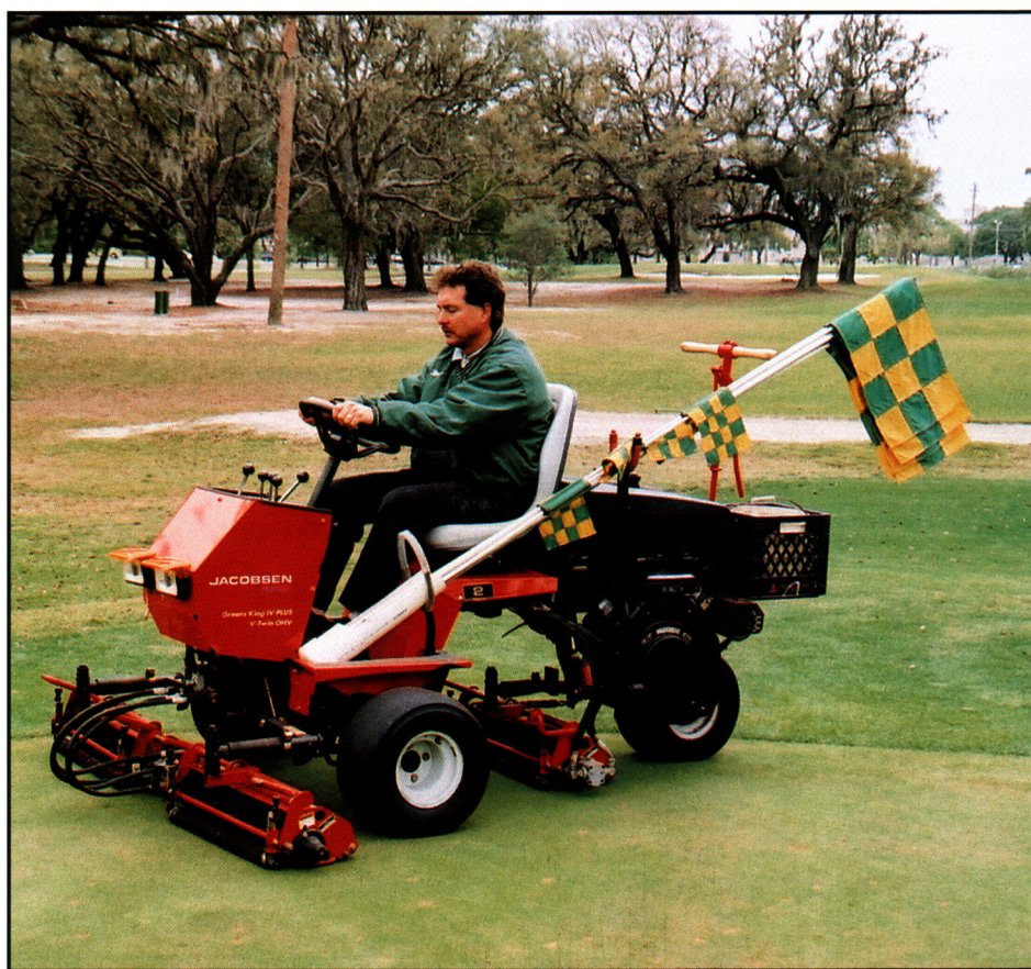
Jim Torba, golf course superintendent at the University of South Florida Golf Course (Tampa, Fla.), uses some creative ingenuity to combine routine jobs to compensate for limitations in resources. Simple modifications to a triplex putting green mower result in the ability to make mowing multi-tasked.
