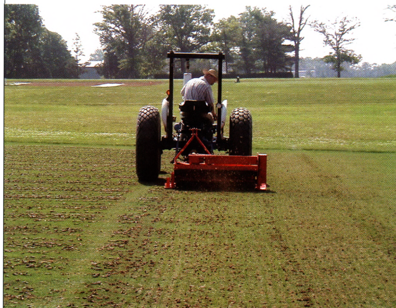
Seeding in the research plots was accomplished by aeration, vertical mowing, application of chemicals, and broadcast seeding. Plots were aerated to ensure good seed-to-soil contact during the seeding process.
