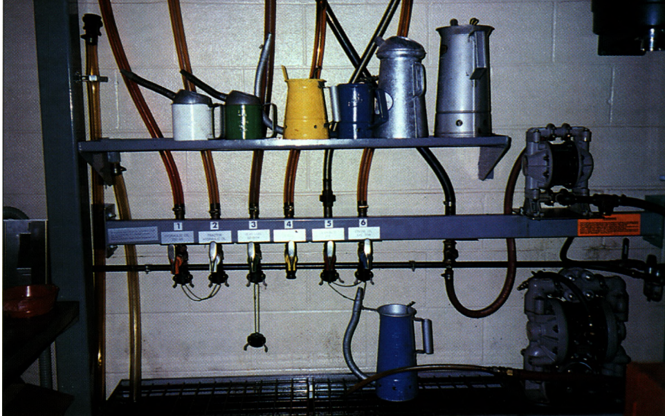
Bulk oil dispensing can be clean and efficient. Oil is dispensed from six steel drums. A drip trough catches any spillage.
