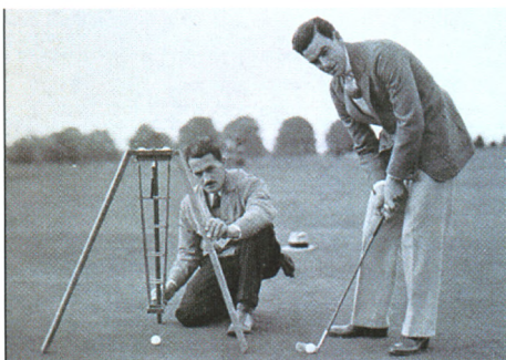
In 1933, Johnny Farrell (right), 1928 National Open Champion, and Dr. Fred Grau, Green Section National Director, tested the putting qualities of grasses at the Arlington turf garden research plots. A mechanical putter was used to minimize the human factors within the test.
