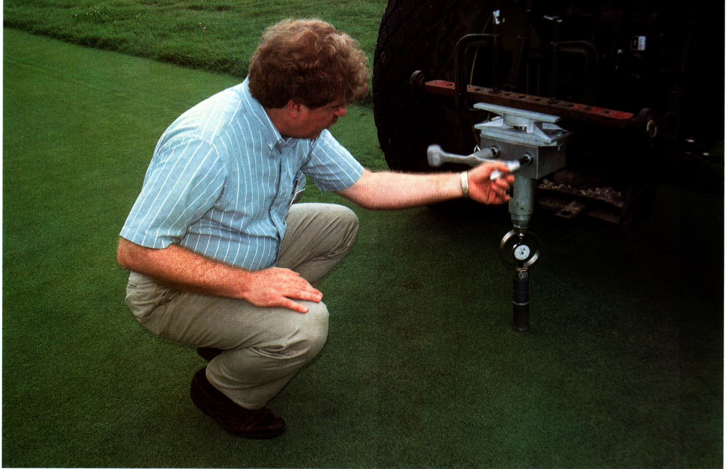
Michigan State University researchers adapted a California Bearing Ratio (CBR) testing device to measure in the field a putting green's soil strength against failure under compression. The CBR device was mounted to a tractor, and a plunger was pushed into the ground with a jack. A load cell with digital readout measured the force on the plunger or the pressure required to deform the putting green surface for each 0.01-inch displacement.
