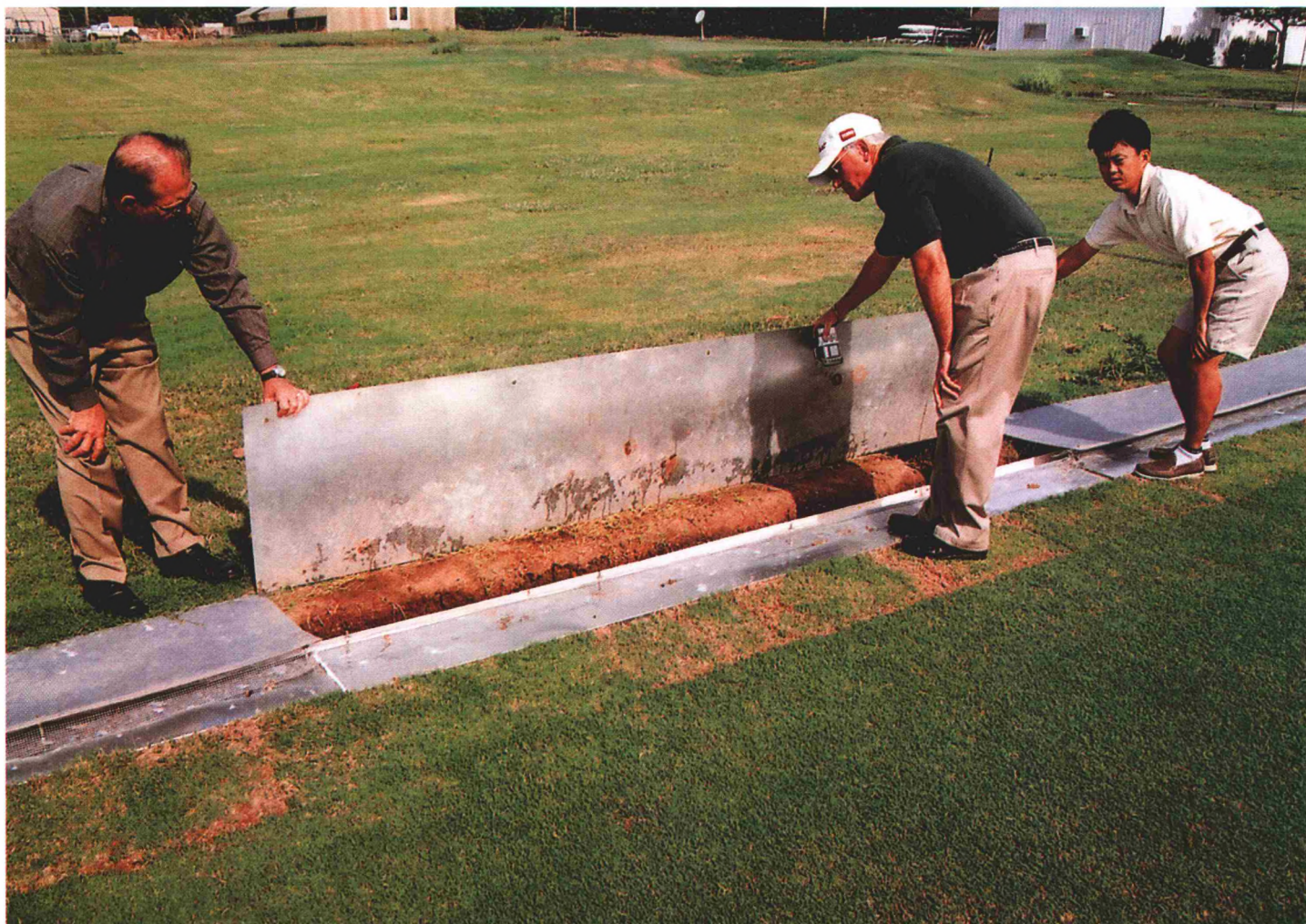
Covered troughs collected runoff water from each plot and channeled it through calibrated Parshall flumes by gravity flow.
