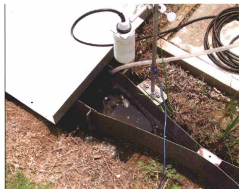
Ultrasonic modules (ISCO 710) mounted over each Parshall flume used ultrasonic reflection to measure water levels and flow rates every five minutes for 60 minutes.
