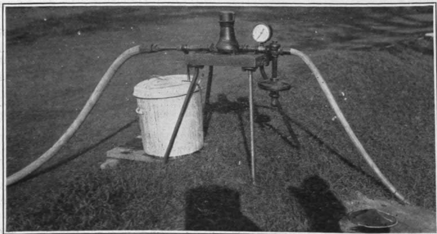
Figure 1.—Proportioning machine for regulating the strength of a solution.
