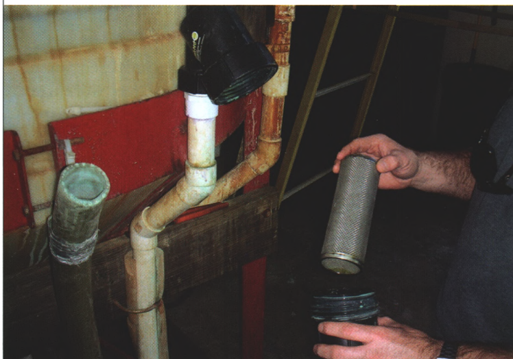
In-line filters are installed in both the tank's fill and discharge lines. Plugged nozzles in the sprayer are a thing of the past.
