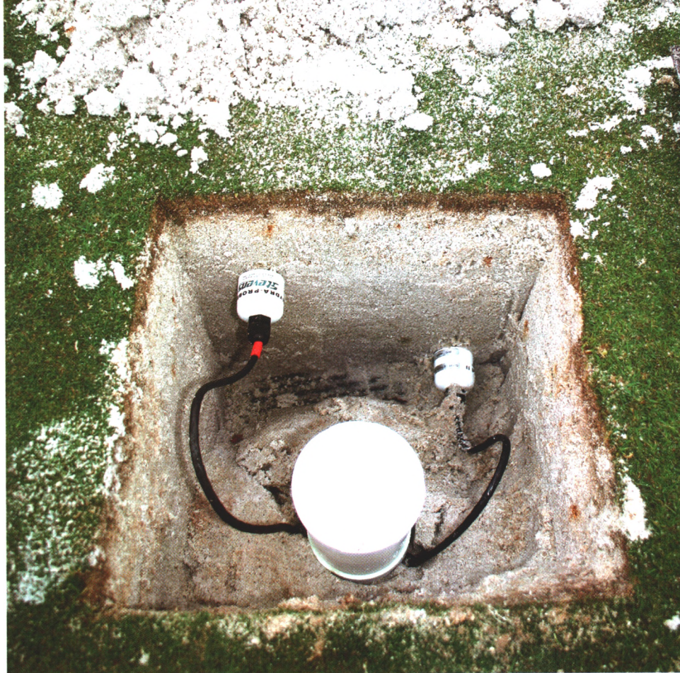
An integral part of the wireless rootzone monitoring system is the node, probe, and sensor unit. Four of these units are installed in the experimental green to monitor soil moisture, soil temperature, and electrical conductivity (salts). The probes are installed 4 inches and 10 inches below the surface.
