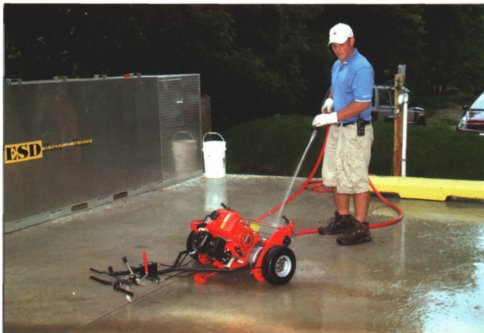
Make sure your chairman knows about your efforts to be a good steward of the environment. Here, clippings and other debris are removed from the wash water and are degraded. The water stays in the system and is recycled.
