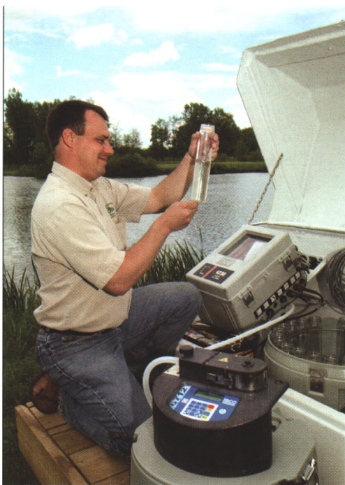
Agricultural engineer Kevin King examines discharge water from a turfgrass system in central Ohio as part of a research program designed to assess how land uses and management affect water quality. This research is funded, in part, by the USGA's Turfgrass and Environmental Research Program.
