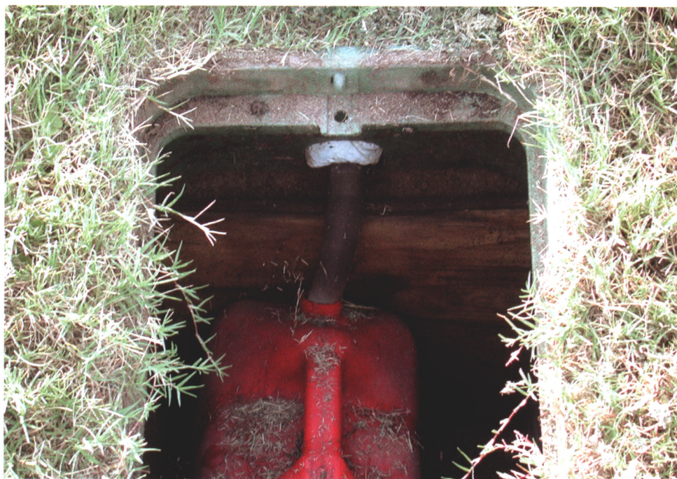
Upon closer inspection, the collection vessel is simply a 5-gallon gas can built into a wood-framed box. The plastic tube that drains into each gas can is attached to the drainage hole of each 70-gallon cattle waterer, which is buried to ground level. Each collection vessel is emptied once per week, unless sufficient rainfall occurs to require additional collection.
