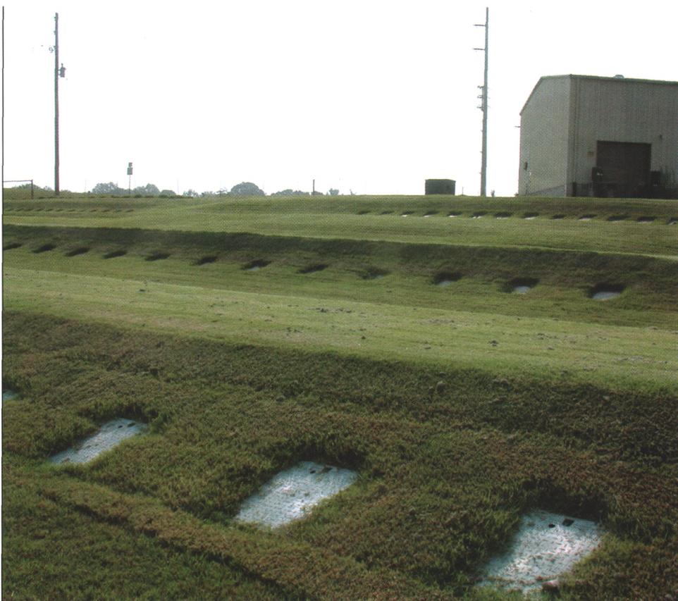
The lysimeter research facility at the Auburn University Turfgrass Unit consists of four sets of 16 lysimeters each. Each lysimeter drains completely into a collection vessel. The collection vessels are housed under the valve boxes shown in the photo foreground, and the lysimeter is built above it.
