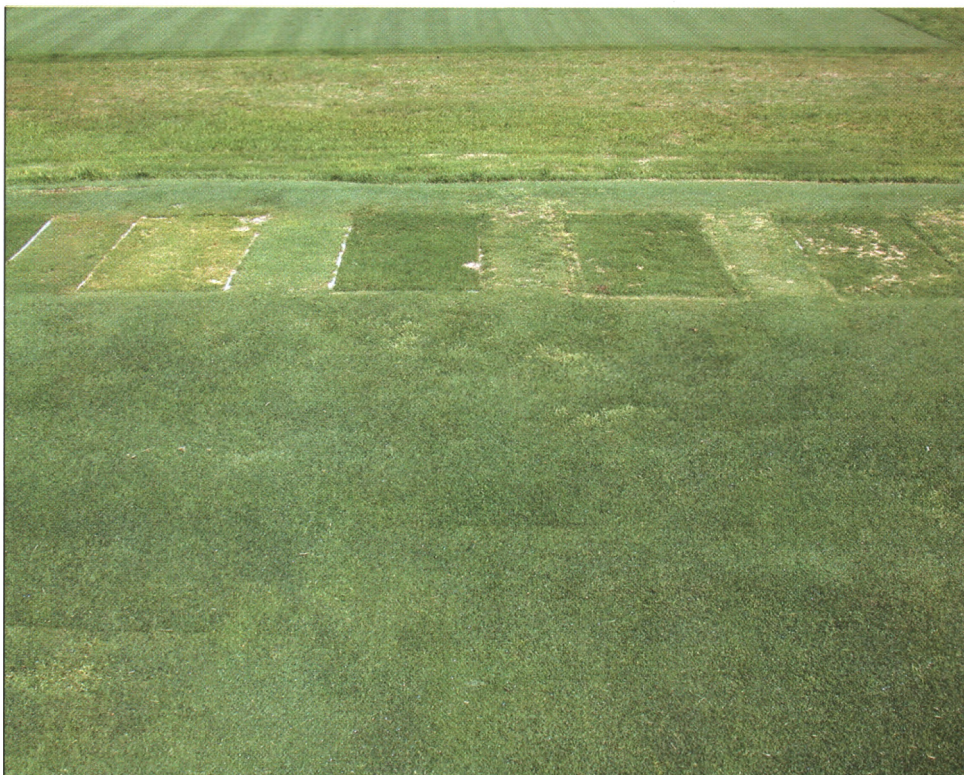
An example of the first-generation lysimeters that were built prior to the switch to plastic cattle waterers. This top view shows four individual lysimeters, each of which drains into a collection vessel.
