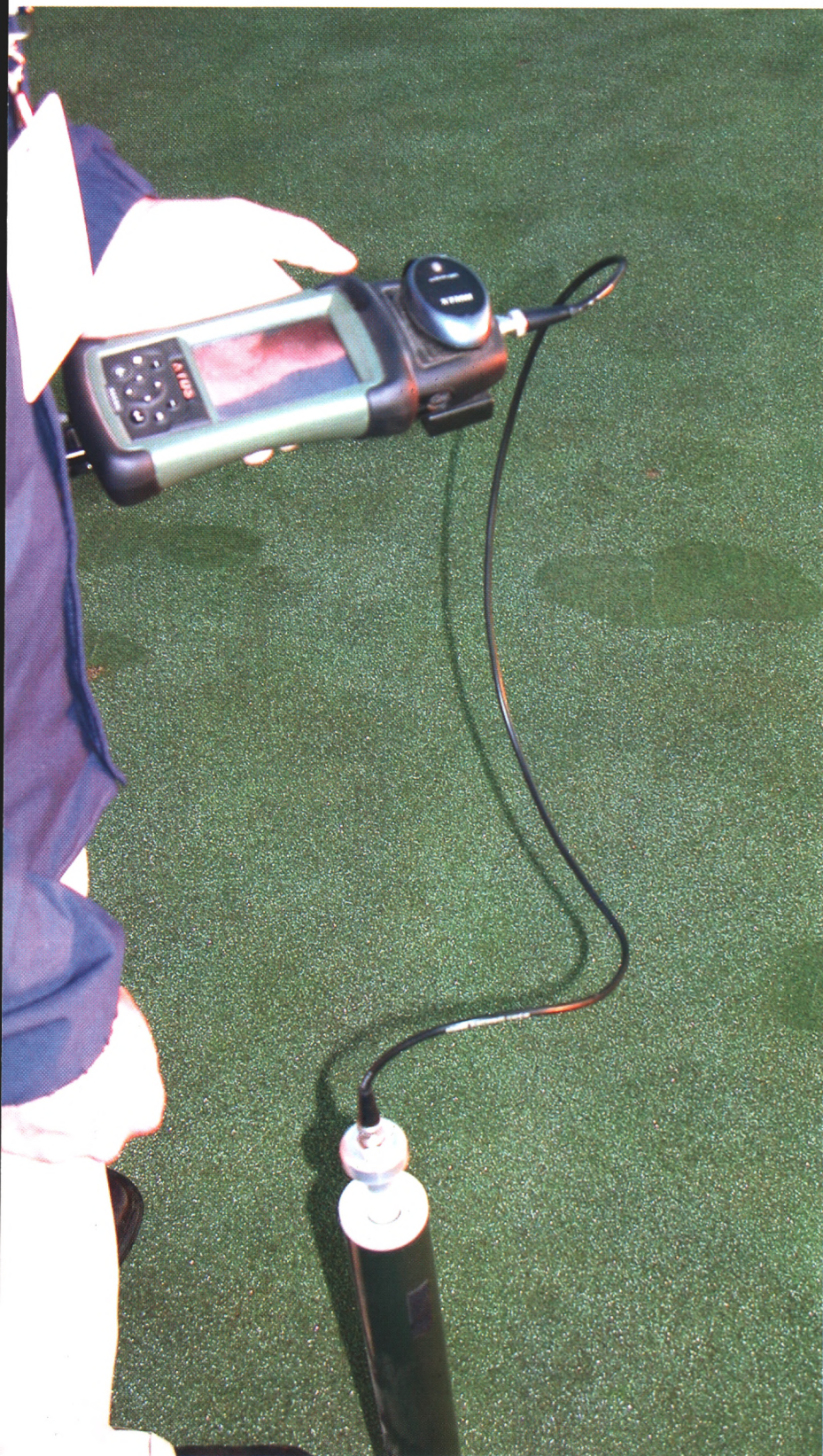
A handheld PC is connected to the slide hammer to record data. The added GPS receiver correlates the location of each data collection drop.
