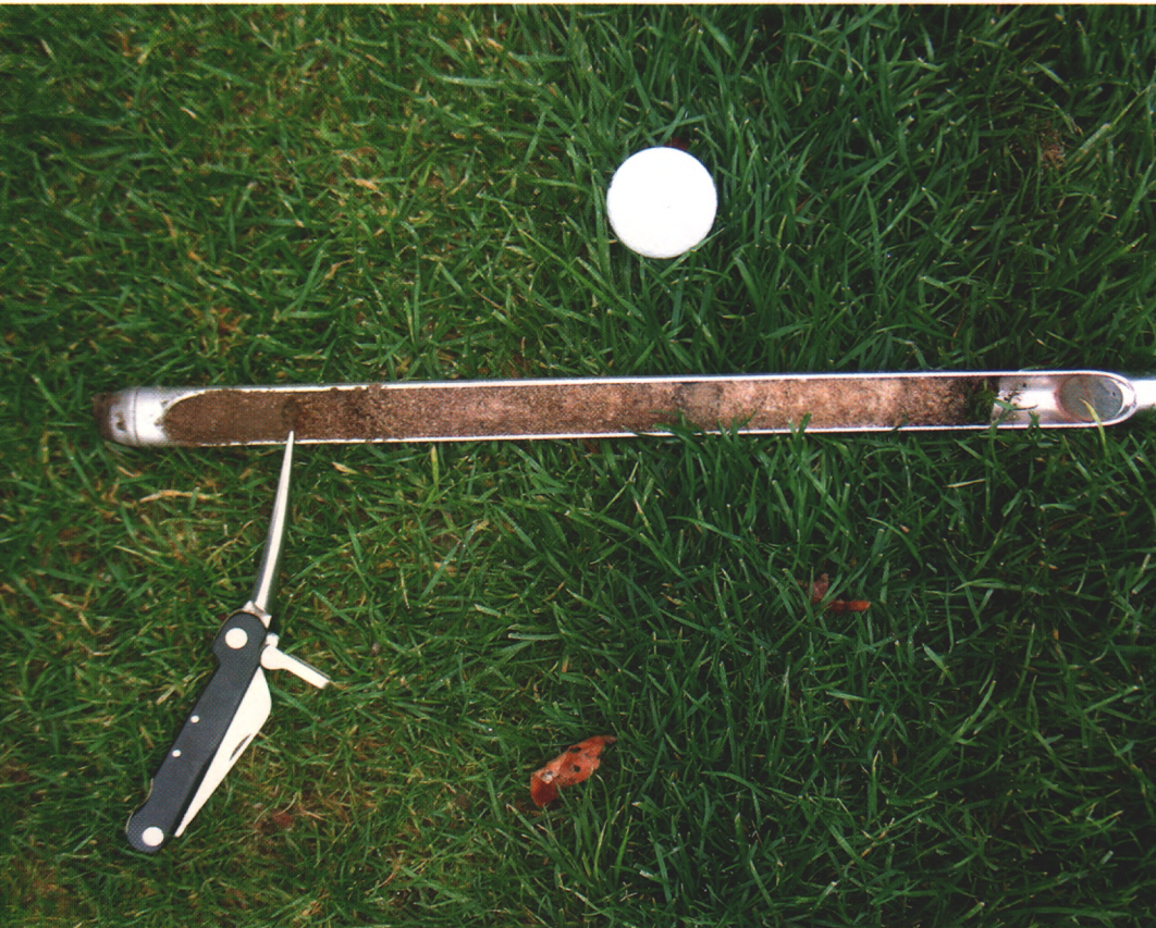
Years of sand being blasted out of bunkers created a droughty, infertile soil that was not capable of supporting healthy turf.
