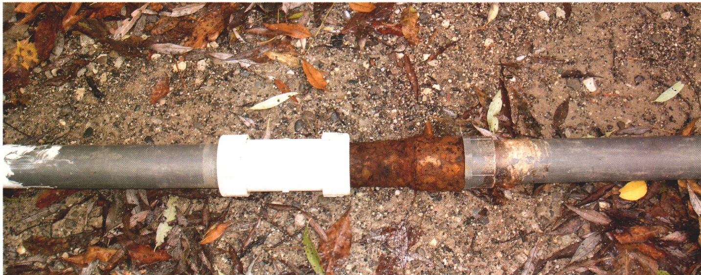
Corroded old pipes were no longer capable of providing adequate hydraulic flow, so coverage and turf performance suffered.
