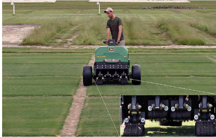
A modified Cady traffic simulator was used to apply traffic once per week during the study period.
