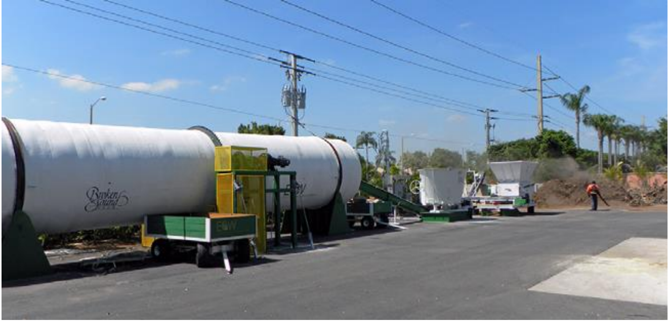
The in-vessel composting equipment is in place and in full operation at Broken Sound Club. At far right, organic debris from the two golf courses is stockpiled and then shredded before being combined with the clubhouse food waste that is then fed into the composter.
