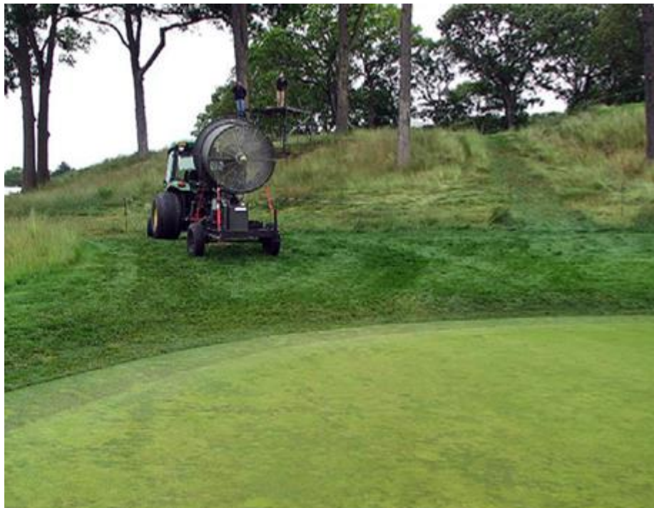
Fans on portable trailers offer flexibility to improve air movement at many green sites.
