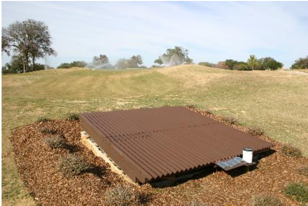
Structure housing filters and test equipment with experimental green in the background. Drain lines from the green enter this structure and are connected to the filters located inside.
