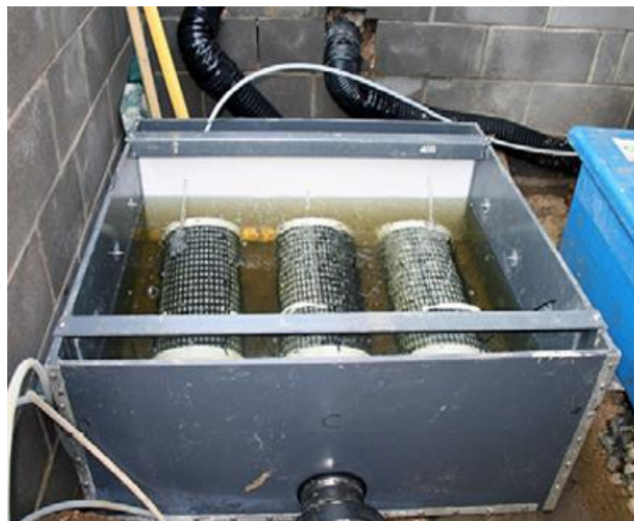
Various filter materials are being tested for their efficacy to remove nutrients (N and P) and pesticides (chlorothalonil, mefenoxam, and propiconazole) from drain
