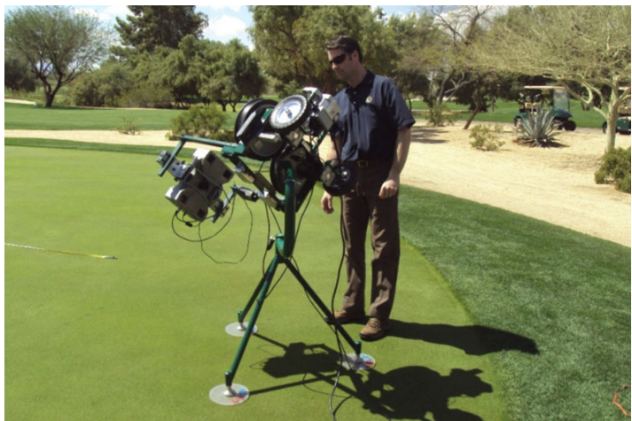
A modified baseball pitching machine was used to fire golf balls into the turf with a range of speeds, spins and angles.
