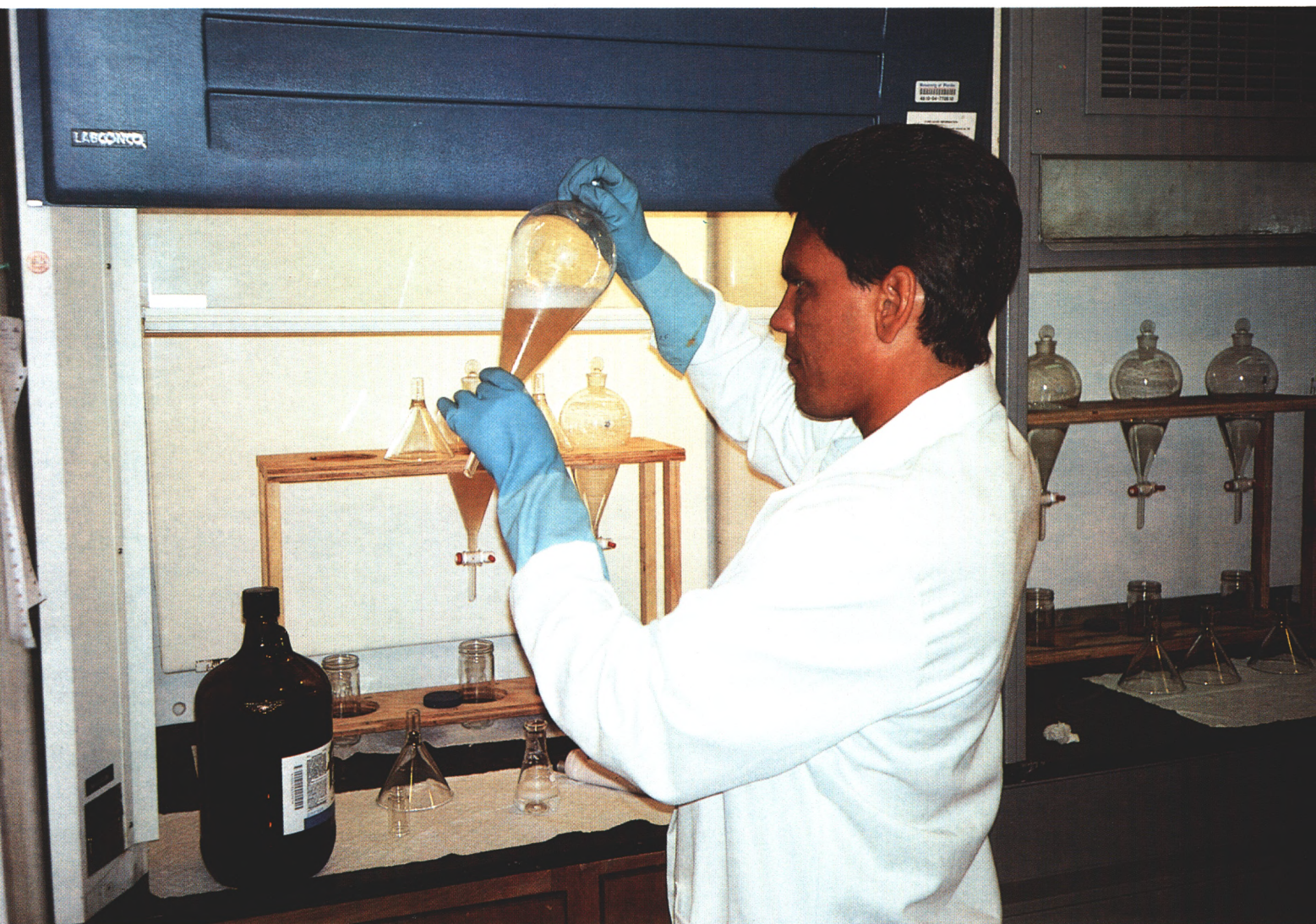
Pesticide was extracted from clippings, thatch, soil, and percolate water for analysis in the Everglades-REC pesticide lab.
