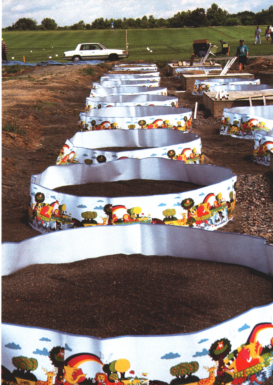
Inexpensive swimming pools provide a unique and useful means of creating large lysimeters.
