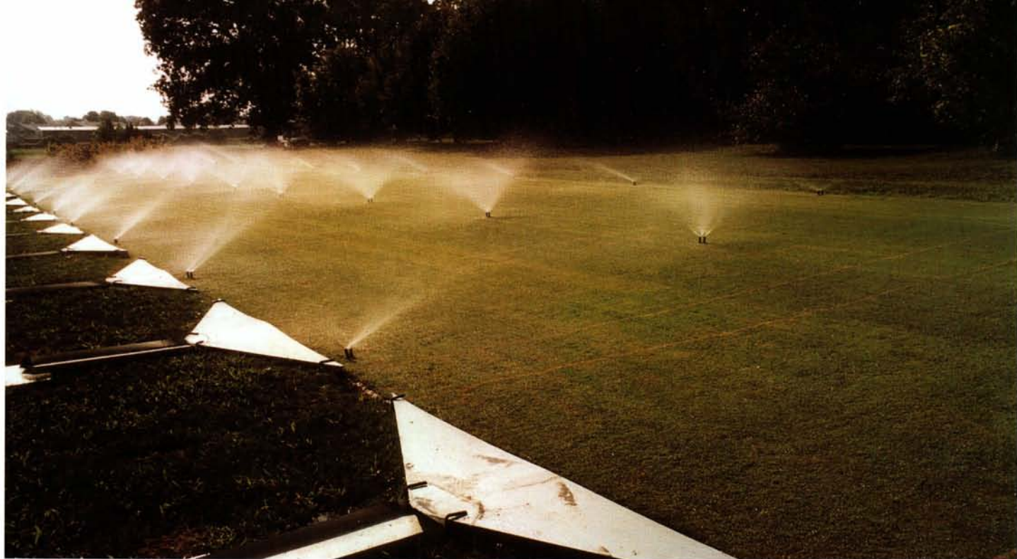
Runoff plots with a 5% slope were constructed at the University of Illinois to study the effects of post-application irrigation and clipping management on runoff of pesticides of varying solubilities.
