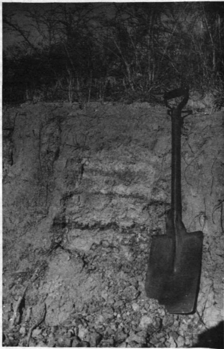
Plate 12: STRATIFIED SEDIMENTS IN ALLUVIAL INFILL NEAR SECTION 12
