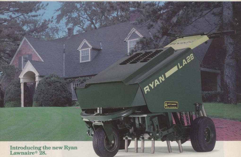
The revolutionary Lawnaire 28 combines the technology and precision of golf course aeration with the demands of lawn maintenance. Its reciprocating, crank mounted tine arms feature a vertical coring action similar to larger Ryan aerators. Tines penetrate straight in to a depth of  $2\frac{1}{2}$  inches, and come straight out. The results are a more professional-looking job, better root development, greener lawns, and more satisfied customers.
