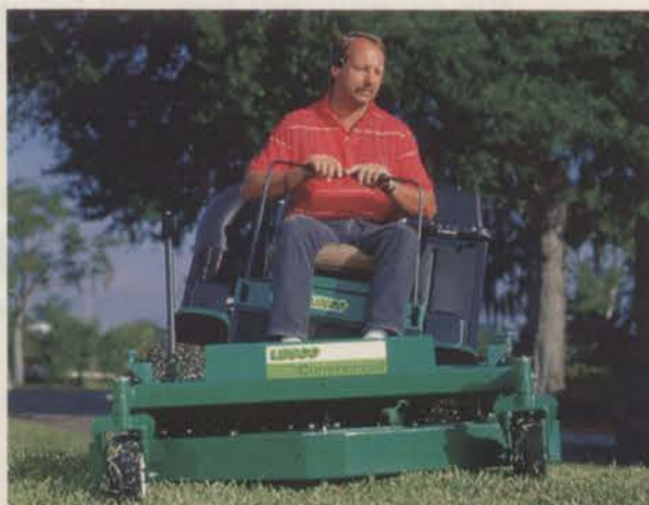
The LESCO 52 Commercial features front-to-back and side-to-side deck articulation.
