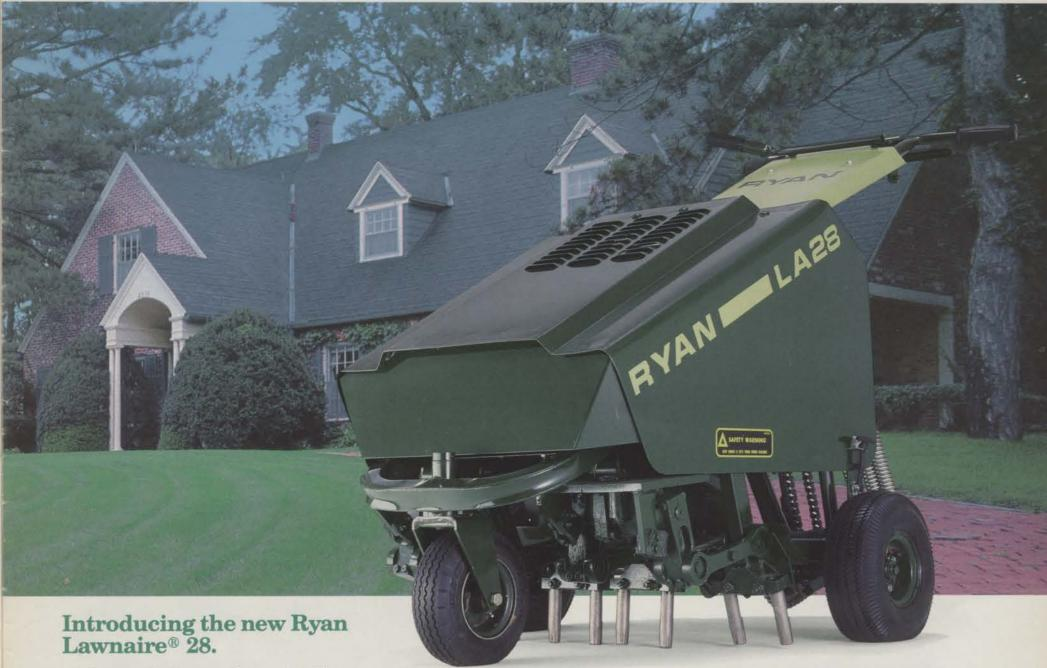
The revolutionary Lawnaire 28 combines the technology and precision of golf course aeration with the demands of lawn maintenance. Its reciprocating, crank mounted tine arms feature a vertical coring action similar to larger Ryan aerators. Tines penetrate straight in to a depth of  $2\frac{1}{2}$  inches, and come straight out. The results are a more professional-looking job, better root development, greener lawns, and
