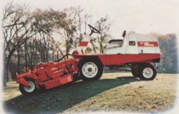
Cutter deck tilts up and down for mowing gullies and bank edges.
