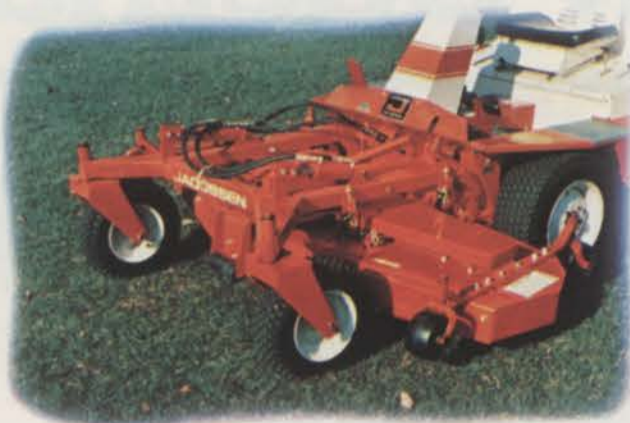
Front wheels support cutter deck for super stability.
