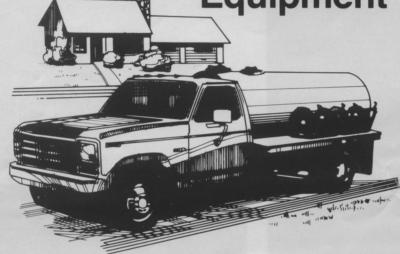
Rugged Minnesota Wanner truck, trailer and skid mounted sprayers meet lawn care professionals' most exacting specifications. Single or multiple compartment tanks range in size from 65-1500 gallons fabricated from stainless, mild steel or polyethylene, with mechanical agitation available to provide optimum chemical mixing. We manufacture a complete line of sprayers, pumps, controls, and turf care accessories, all with Minnesota Wanner quality and dependability!
