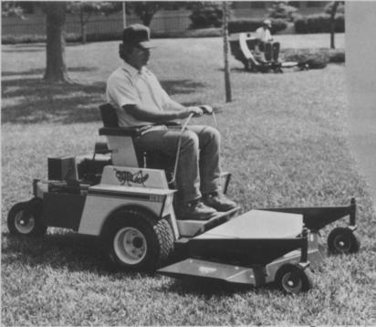
**Easy Operation**–Two Operating Levers Do It All... Control Ground Speed and Direction.
