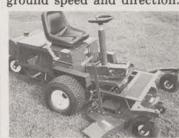
The steering wheel increases or decreases the individual wheel speed to provide the steering.
