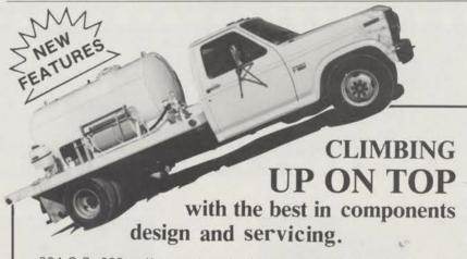
304 S.S. 600 gallon tank • dual stage centrifugal pump (100 GPM or 200 PSI) • sparger agitation • PTO drive • 12 volt electric reel • low to the ground work platform • Options: 5 gallon hand rinse tank & bracket • SOLO 425 (475) Knapsack Sprayer and stand
