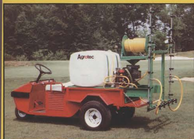
100 gallon skid #ASD 1054 (shown with reel kit #EK0385 & 15' boom #EB3158)
