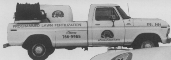
300 gallon fiberglass tank jet spray agitation
