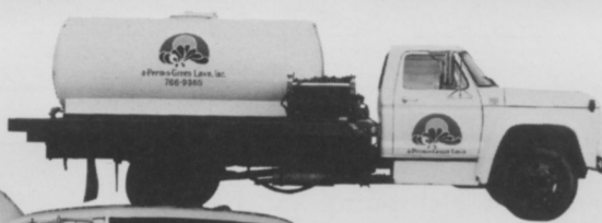
950 gallon fiberglass tank jet spray agitation
