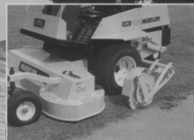
Coulter-type edger eliminates the need for conventional hand edgers.
