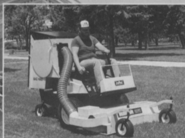
The new "BacVac" grass vacuum attachment has a 15-bushel capacity.
