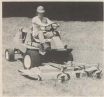
gas engine rated at 23 hp, with 39 foot-pounds of torque at 2500 rpm.
