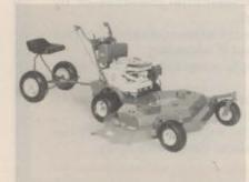
trol independent power and brake on each traction wheel. Also, the cutting width and optional rider attachment provide equal productivity with tractor-mounted mowers at about half their cost.
