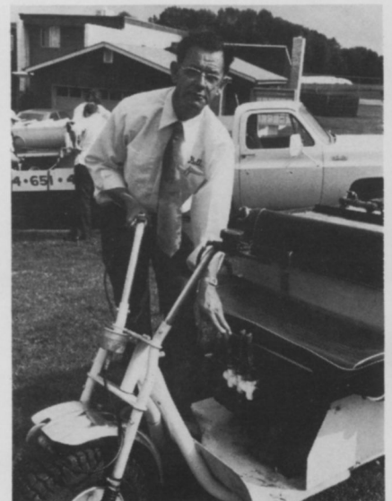
Chem-Trol owner Bill Shearman points out three nozzle controls which release a spray solution at the back of his specially-designed spray unit.
