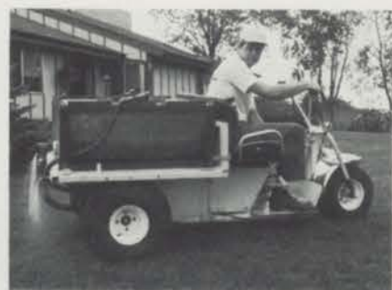
Dave Feest operates Chem-Trol's three-wheel spray unit. It can cover a 6,000 square-foot area with chemicals in five minutes.
