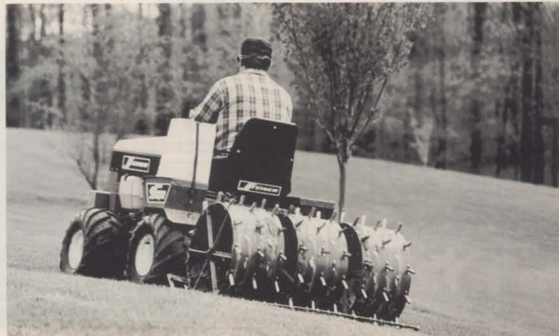
This pull-behind aerator is one of many different sizes and styles of turf aerator.
