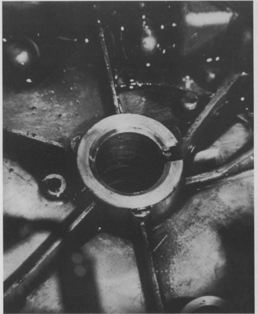
Scoring from dirt inside engine
