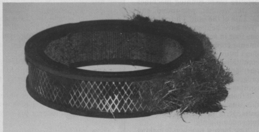
Improperly maintained cleaner element
