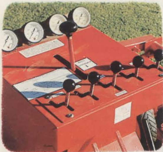
The gauges monitor hydraulic pressures of reel mowing systems. All testing is done under varying operating conditions to assure product excellence.
