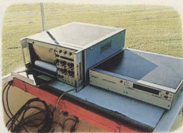
Engine and reel RPM's are monitored by the readout device on the right and fed to the strip chart recorder on the left which continuously prints out data.
