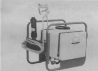
The sprayer is completely selfcontained with a poly tank, trigger grip spray gun with adjustable nozzle and 15 feet of hose. The electric diaphragm pump is rated at 45 psi and up to 2.8 gpm. The sprayer itself delivers a straight stream up to 25 feet.
