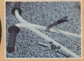
Chip-resistant powder coat epoxy paint is baked on for longer lasting finish.
