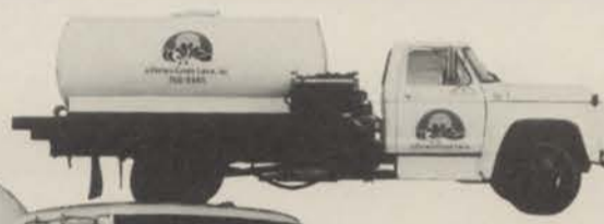
950 gallon fiberglass tank jet spray agitation
