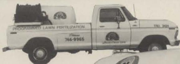
300 gallon fiberglass tank jet spray agitation
