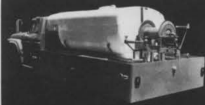
Model #PC 1200 fiberglass tank equipped with fiberglass pump cover, Model #D 200 gallon mixing tank shown mounted on a custom truck body by Strong Enterprises.
