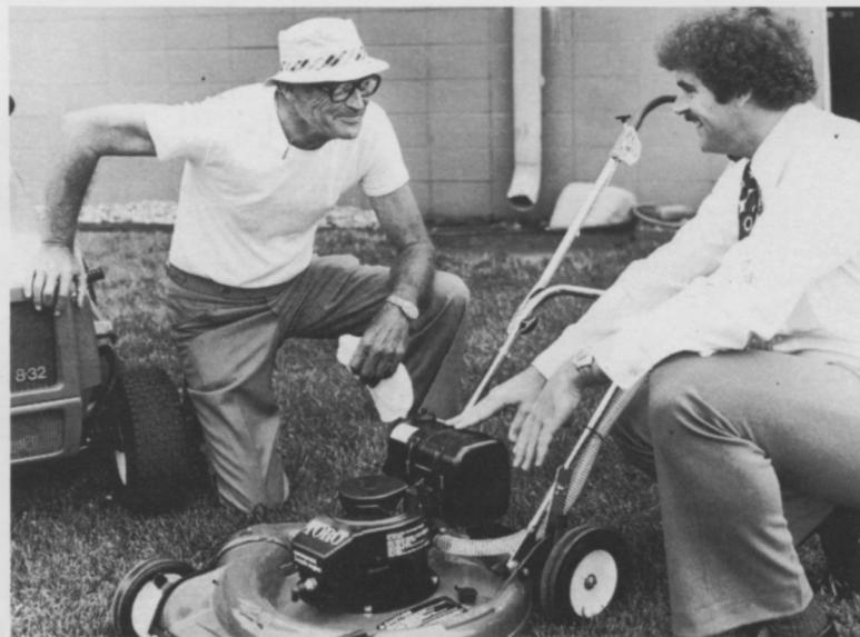
Paul McGuire of McGuire Lawn Care, St. Paul listens to Toro's Bill Albert describe the features of the company's new two-cycle heavy duty rotary for commercial use: remote air cleaner for longer engine life and five-quart fuel tank.
