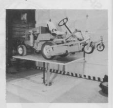
A two inch steel safety leg with an automatic latch will hold up the table in the event of a hydraulic or electrical failure and a pressure relief valve built into the hydraulic pump provides overload protection. The platform is made of safety tread steel plate and is painted O.S.H.A. yellow.
