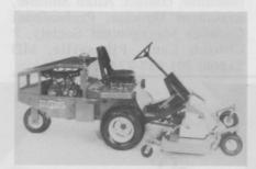
Steered by a single wheel for a shorter turning radius, the tractor also features assist brakes used for either right or left drive wheels for a complete zero turning radius. The side drive wheels are activated hydrostatically by hydraulic pump along with a differential. Other available attachments include a 60 inch V-type plow, a 60 inch angle-type blade, 60 inch rotary broom, a two-stage snow thrower and a cab for the operator's comfort.
