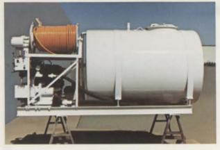
Now you can utilize your pick up truck with an easy on and off full feature sprayer. This system also has high volume agitation capable of spraying IBDU, Powder Blue, and wettable powders. Powered by a two cylinder 16 h.p. engine this system offers everything the truck systems do including a chemical inductor and two compartments.
