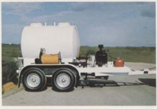
This trailer model offers every advantage a truck has including a chemical inductor and 600 gallon capacity. Powered by a twin cylinder 16 HP air cooled engine you get economy without sacrificing performance.
