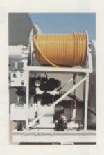
The chemical inductor, pressure gauge and control valves are all conveniently located on stressed steel mesh.
