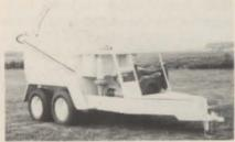
horsepower Wisconsin engine, high pressure Hydro or mechanical agitation, direct and convenient loading from two vehicle, fold down spray turret, four wheel electric or hydraulic brakes, ground level controls and many other features found on their low cost models 300 and 600.
