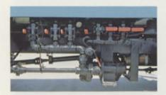
Maintenance is always important to any lawn spray business. Pump and valves are not only rugged and dependable but allow for easy access for operation and maintenance. Note also the convenient location for the intake and output couplers for easy loading and transfering of materials.
