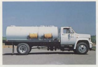
Shown here is a three compartment system allowing the applicator to apply three different mixes by simply moving levers.
