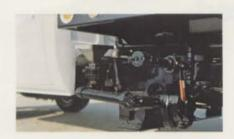
The same high volume pump from the larger systems powers this system. Note the chemical inductor as well as the intake and output couplers are also included. (available also with a 16 h.p. independent power source)
