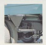
All Professional Turf Systems are available with a chemical inductor. Liquids, wettable powders, and granules can be added directly to your main or auxiliary tank.
