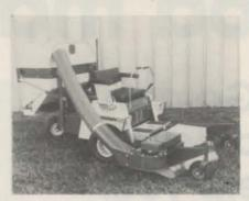
nect of PTO drive for easy attachment of the following options: snowthrower, dozer blade and rotary broom. Two styles of optional grasscatchers mount on the mower offering either lever-actuated self-dumping or slide-out, mesh collection hoppers.
