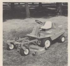
euverable rear wheel steering permits tight trimming trees and under shrubs. Articulated deck suspension allows operators to mow hills and dales and climb curbs when in transit.
