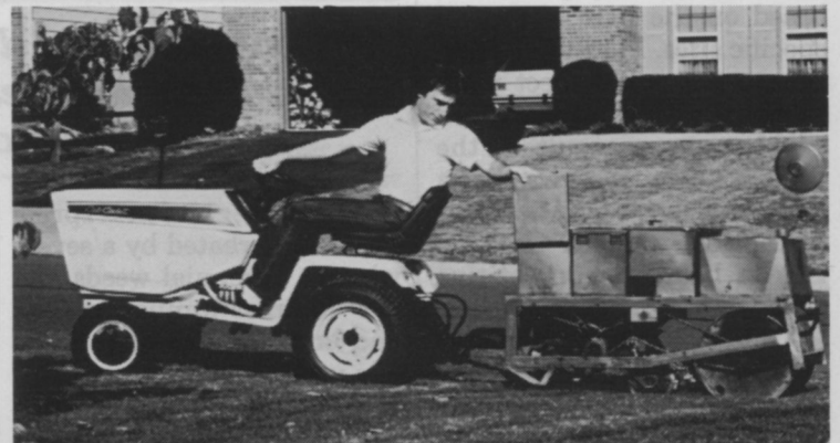
Bailey: Aboard the Seeding Combine made of stainless steel by his company; it aerates, slices, seeds, fertilizes, sprays and rolls.
