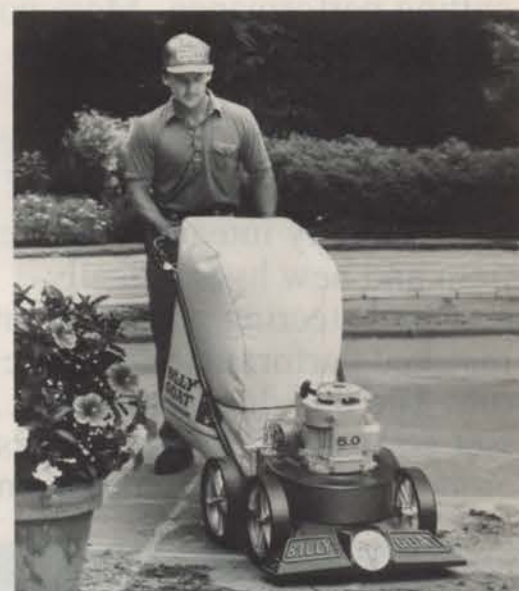
The suction sweeper is used for sweeping up leaves in outlying areas, away from the truck.
