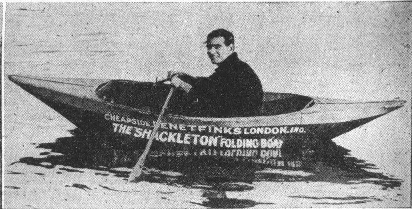
IT FITS INTO A SUITCASE. —Ernest Shackleton in the Shackleton folding boat. The boat can be folded up like a suitcase. As it is made of hide it is absolutely waterproof and weighs a little over ten pounds.
